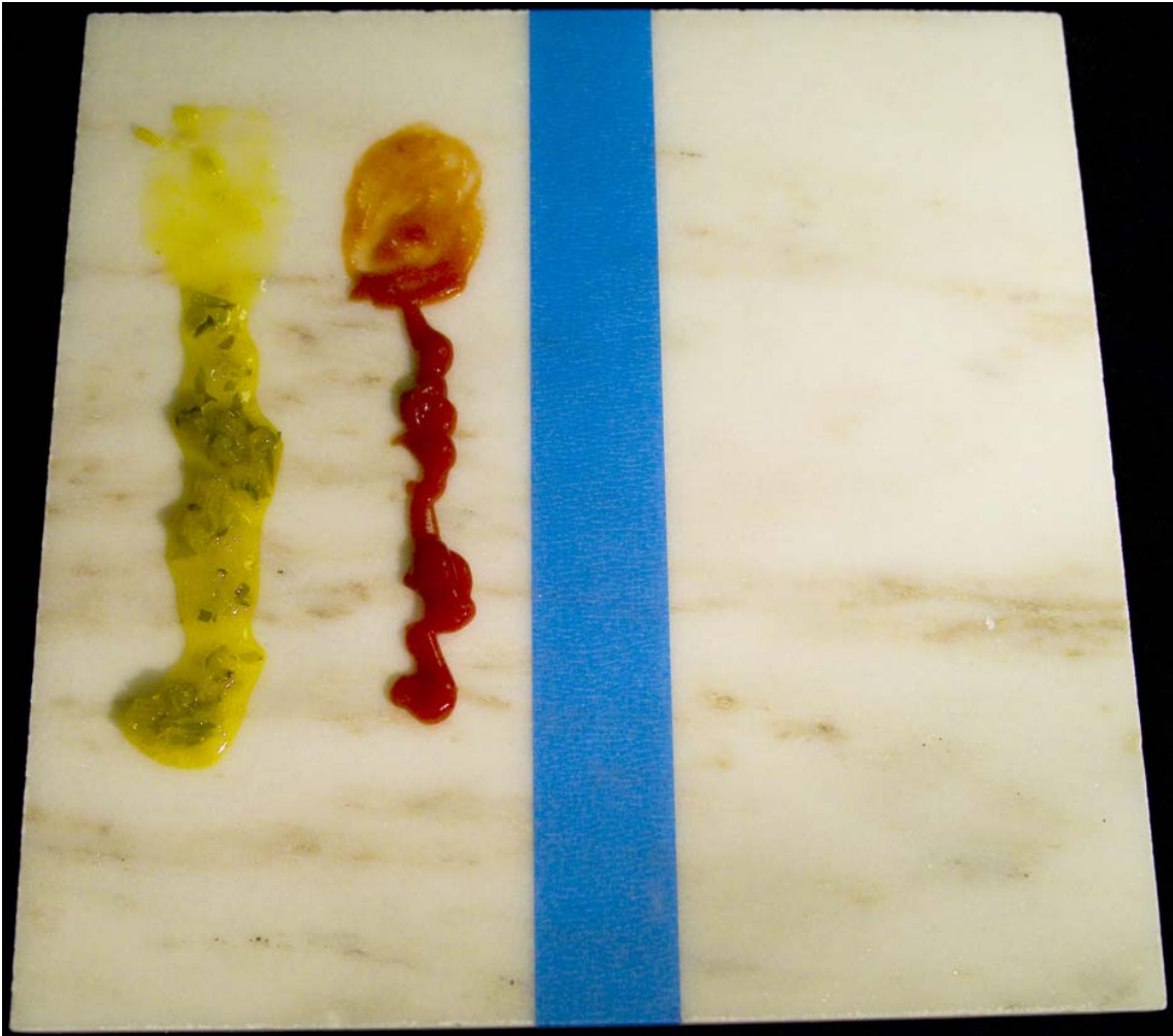
Ketchup and Relish were liberally applied to the sealed surface and allowed to set for 20 minutes. It was then rinsed off with water and the stone was dried.
